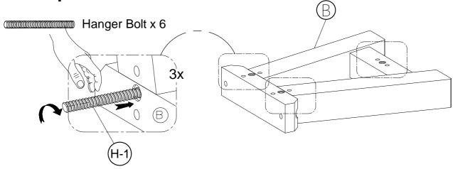
Place both Legs (B) onto a padded, non-marring surface with holes facing up. Insert Hanger Bolts (H-1) into 3 receiving holes per Leg (B) and tighten by hand. Note: DO NOT use any tools to tighten Hanger Bolts (H-1).
