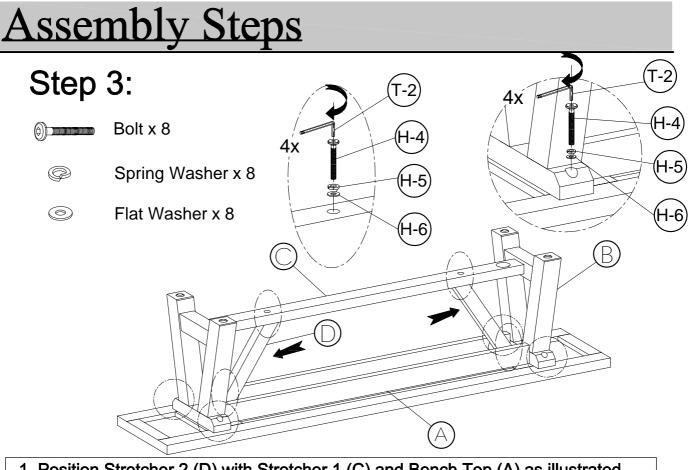
1. Position Stretcher 2 (D) with Stretcher 1 (C) and Bench Top (A) as illustrated. Secure Stretcher 2 (D) to assembly using Allen Bolts (H-4), Spring Washers (H-5) and Flat Washers (H-6), stacking the hardware in the order as shown. Do not yet fully tighten.
